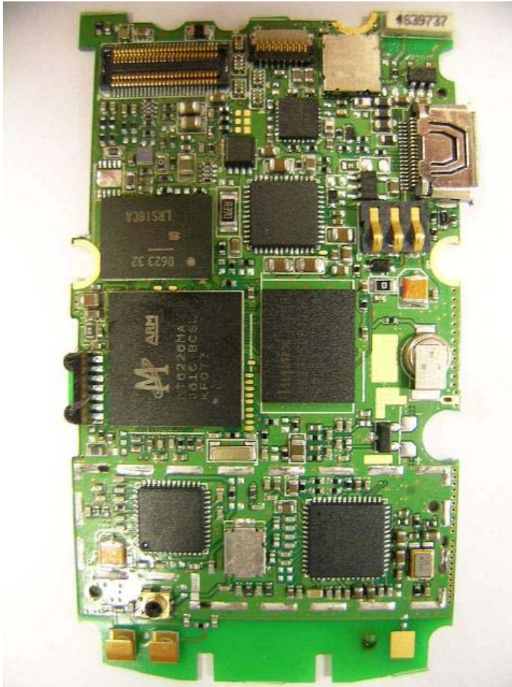
Picture 5: Radio part with the shielding cover removed—1
