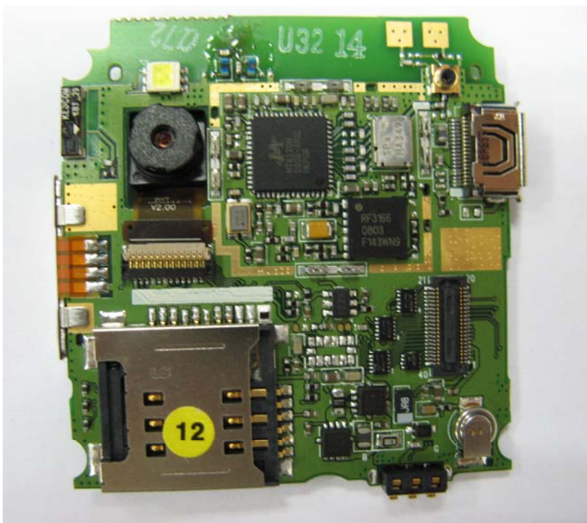
Picture 4: the back view of the PCB with the shielding cover remove
