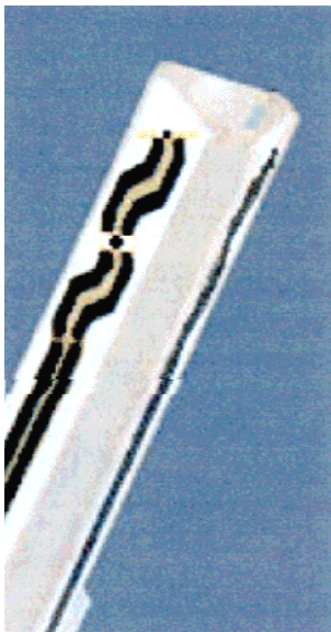
Figure 5. ET3DV6 E-field Probe
