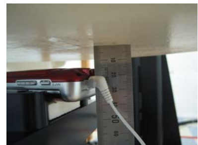
Fig. 19. Body SAR Test Setup with Holster
