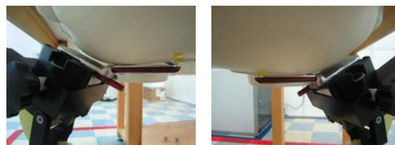
Fig. 17. Head SAR Test Setup
