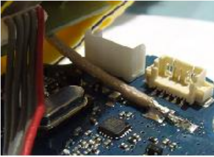
Cable from TNC connector soldered to radio PCB as shown.
