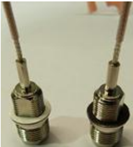
TNC connector for external antenna.
