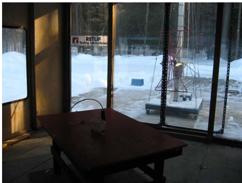
Test Setup, Vertical Antenna Polarization
