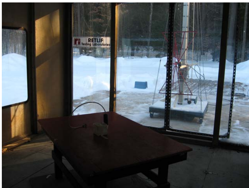
Test Setup, Vertical Antenna Polarization
