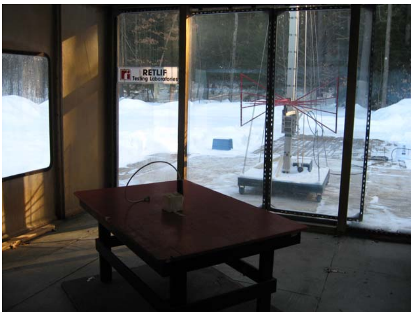
Test Setup, Horizontal Antenna Polarization
