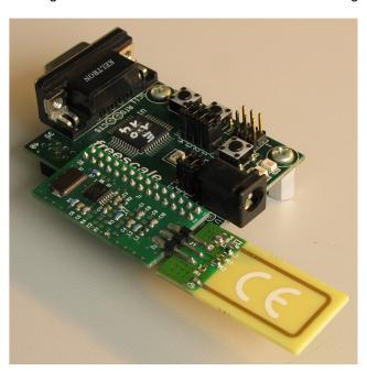
MC33493MODxxx tool can be used to send an RF signal. Some configuration files ("script") are provided to allow one frame transmission to make a link between one MC3493MODxxx kit and a receiver. Each transmission is under user control.
