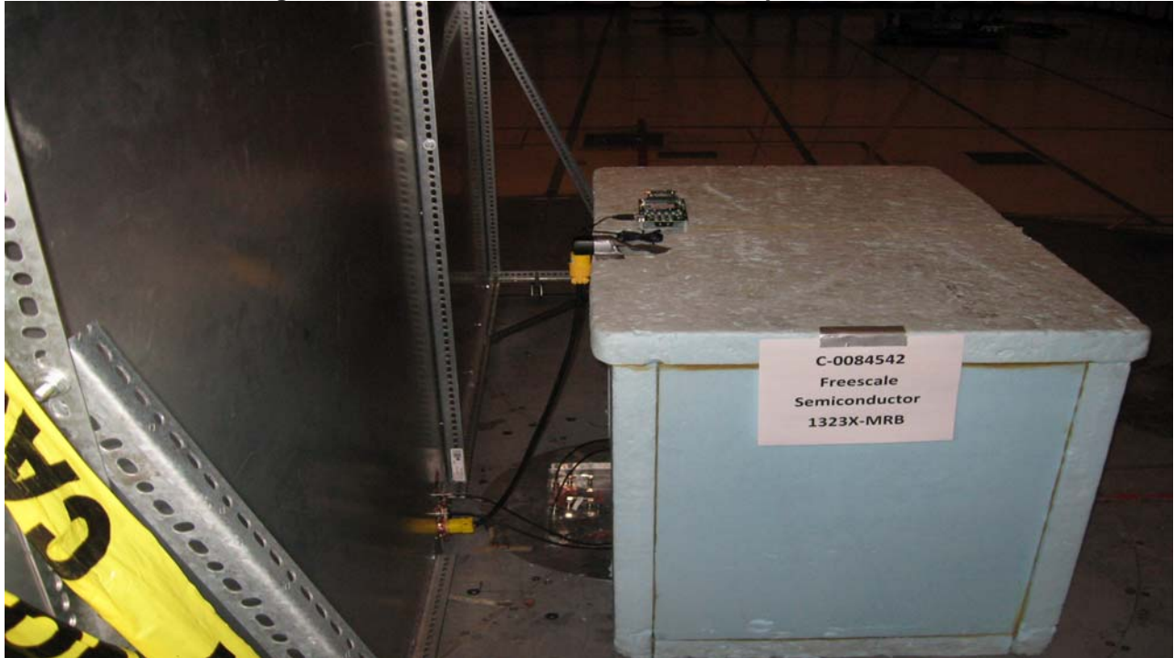
Figure 10 Conducted Emission Test Setup with REM
