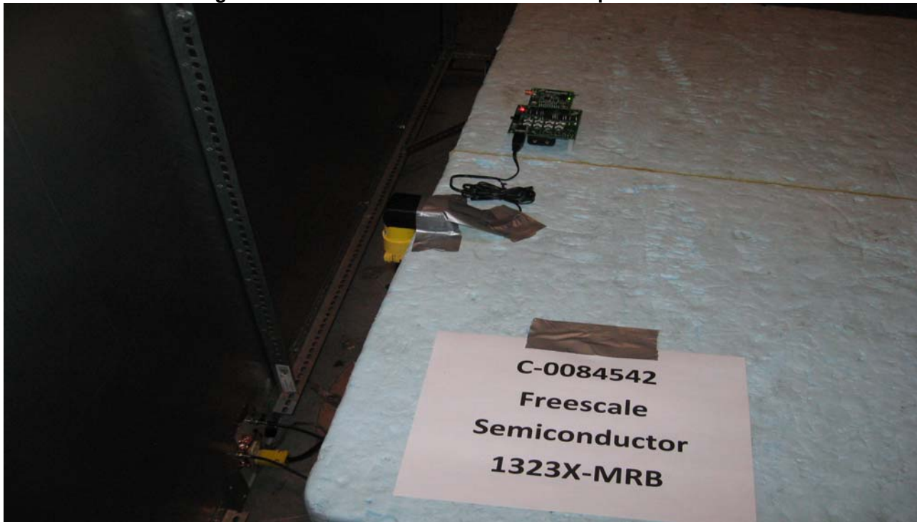
Figure 10 Conducted Emission Test Setup with REM
