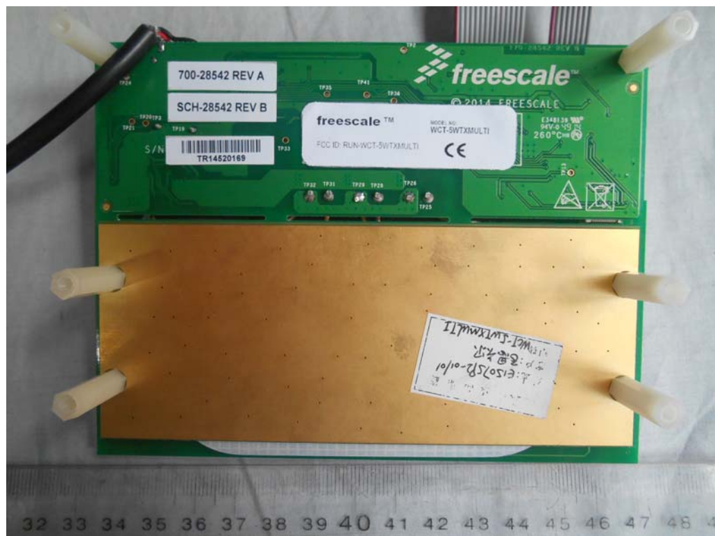
FIGURE 2 A28 MULTI-COIL WIRELESS CHARGER TRANSMITTER (M/N: WCT-5WTXMULTI) GENERAL APPEARANCE (BACK VIEW)
