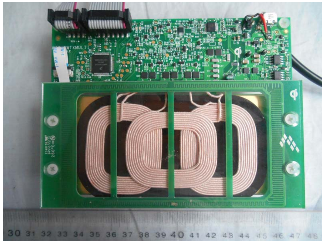
FIGURE 1 A28 MULTI-COIL WIRELESS CHARGER TRANSMITTER (M/N: WCT-5WTXMULTI) GENERAL APPEARANCE (FRONT VIEW)
