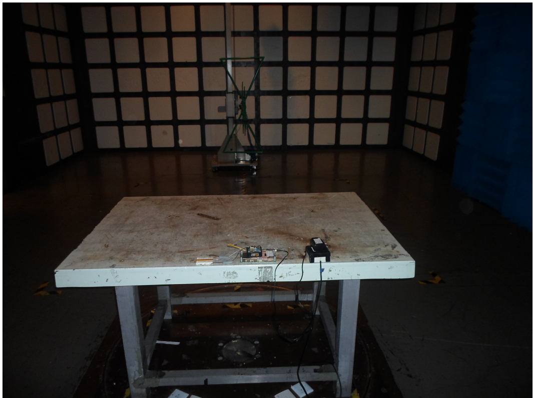
BACK VIEW OF RADIATED EMISSION TEST
