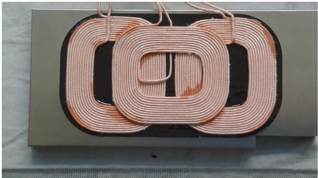
FIGURE 8 QI WIRELESS CHARGING TRANSMITTER (M/N: WCT-5WTXAUTO) COIL
