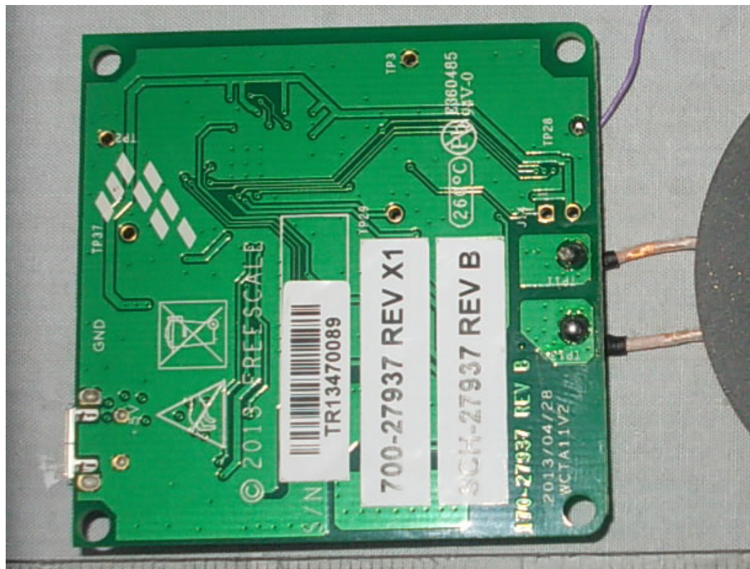
FIGURE 7 WIRELESS CHARGER TRANSMITTER (M/N: WCT-5W1COILTX) MAIN BOARD (SOLDERED SIDE)
