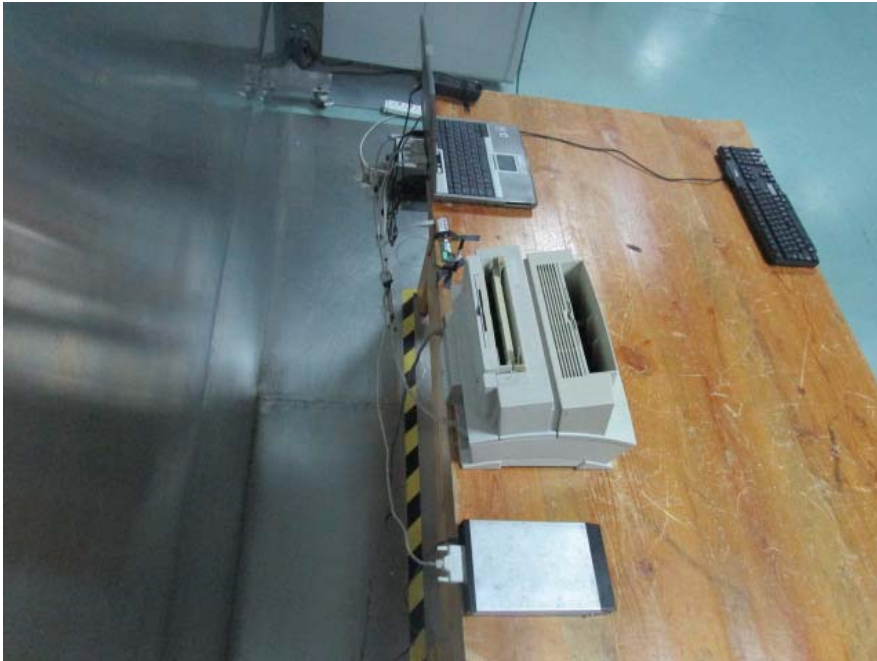
Conducted Emissions – Side View
