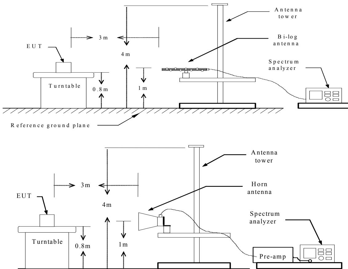
Above 10 GHz shall be extrapolated to the specified distance using an extrapolation factor of 20 dB/decade from 3m to 1.5m.
