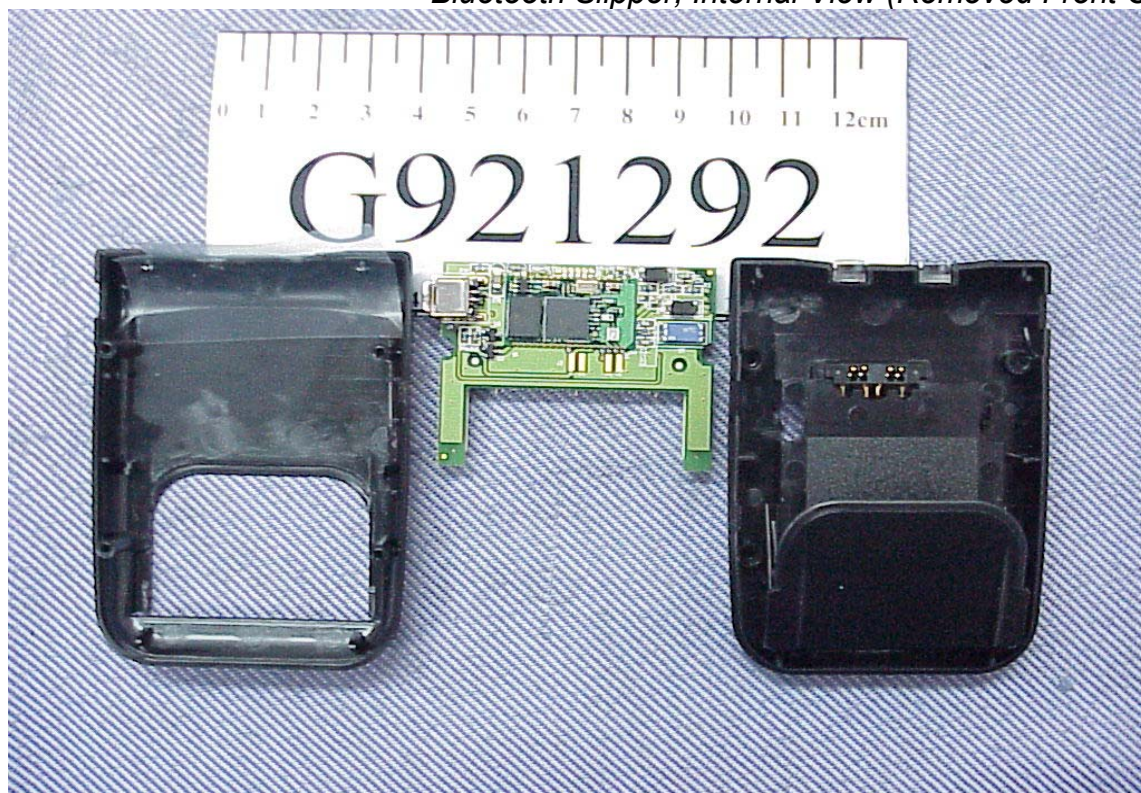
Figure 11 Bluetooth Slipper, Internal View (Removed Front Cover)
