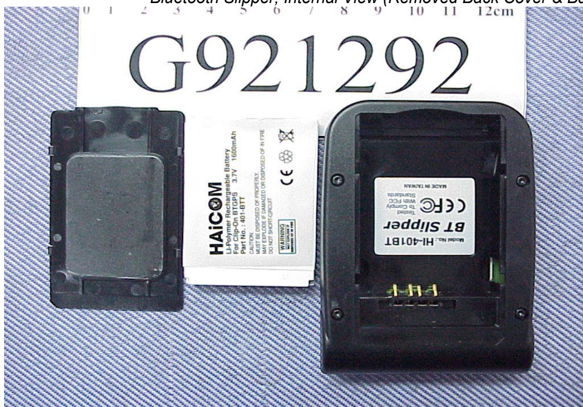
Figure 10 Bluetooth Slipper, Internal View (Removed Back Cover & Battery)
