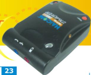
Press " 62 " for automatically enable dial back when GPS location speed mode than 20 km under moving sensor activated mode.
