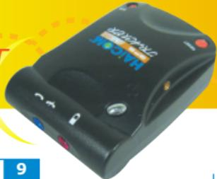
Inside HI-601VT, the GPS module receive satellite signal and transfer the data into standard NMEA protocol data. Then, the GSM module transmit the data in analog voice message via regular communication network (just like calling and talk from one phone to another phone).
