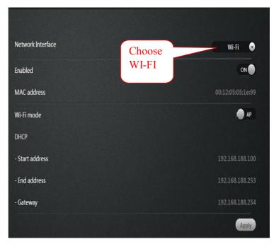
By connected with hot spot can realize the WIFI P2P connections.
