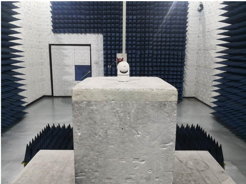
FCC RADIATED EMISSION TEST SETUP ABOVE 1GHZ
