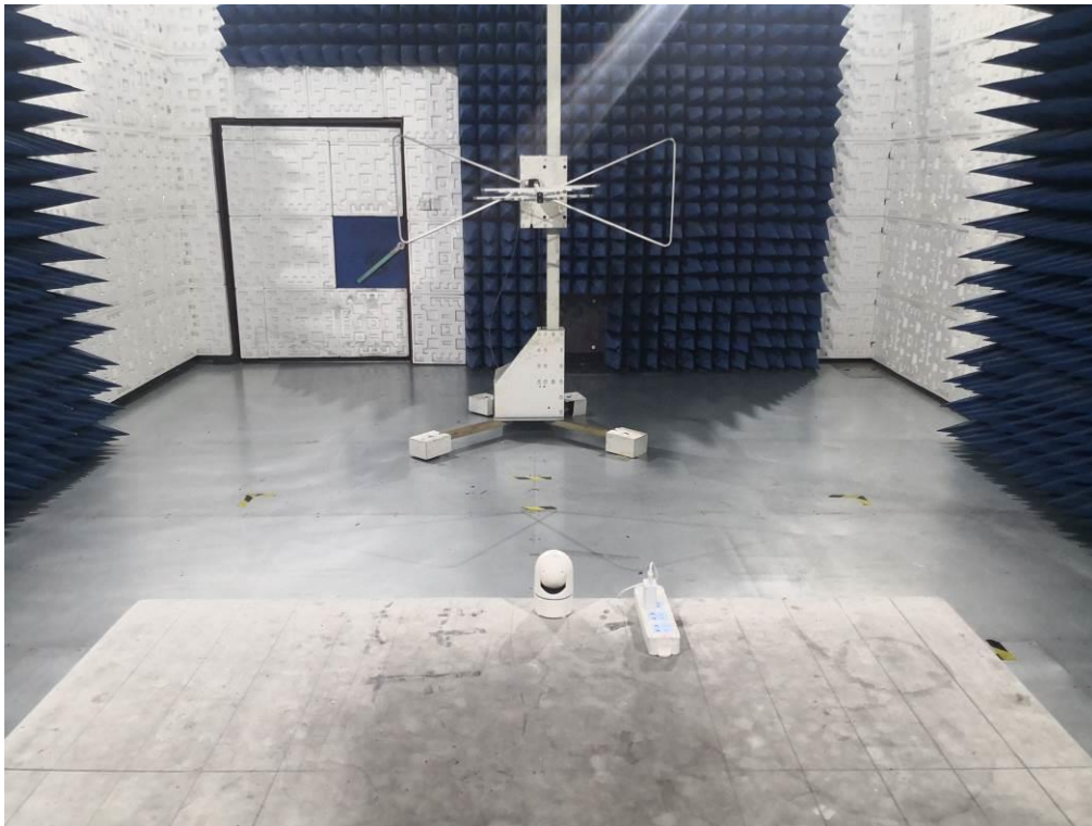
FCC RADIATED EMISSION TEST SETUP ABOVE 1GHZ
