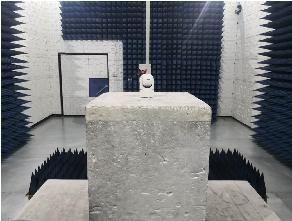
FCC RADIATED EMISSION TEST SETUP ABOVE 1GHZ
