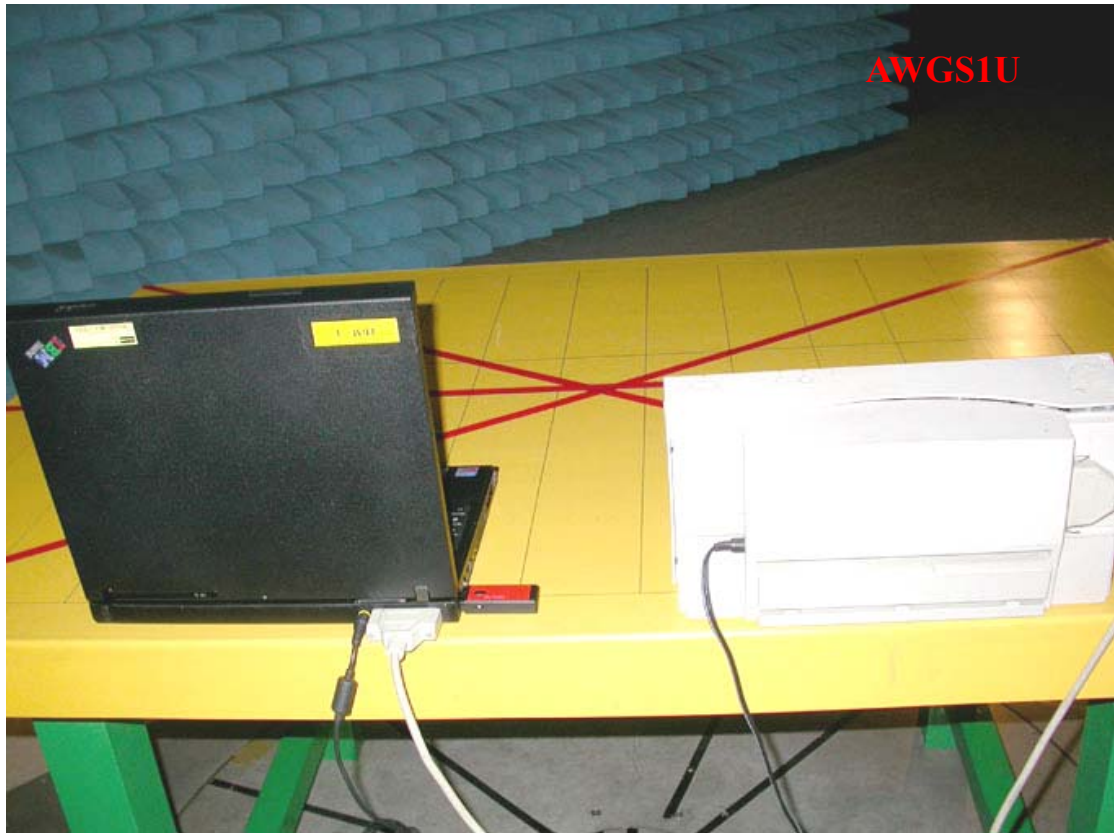
Photo 2: Radiated Emission Test set-up photo
