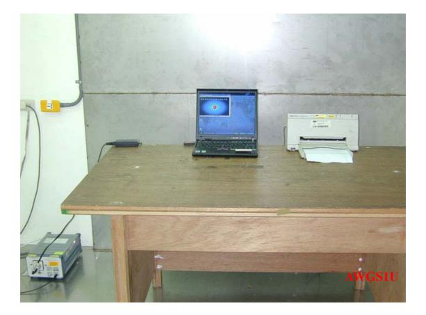
Photo 2: Conducted Emission Test Set-up photo
