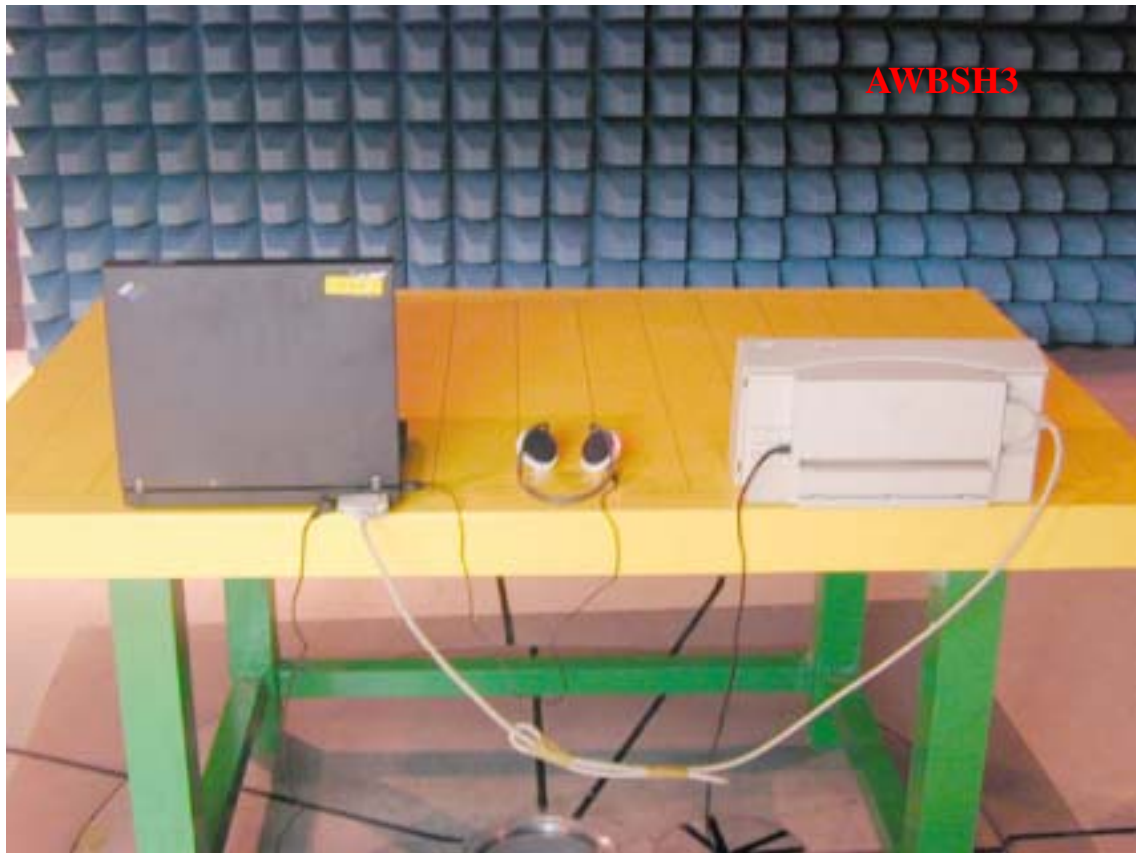
Photo 2: Radiated Emission Test set-up photo
