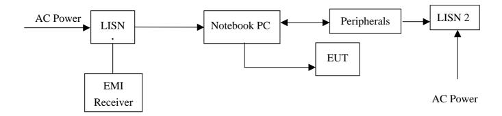
The EUT are connected to the main power through a line impedance stabilization network (LISN). This provides a 50 ohm/50uH coupling impedance for the measuring equipment. The peripheral devices are also connected to the main power through a LISN that provides a 50ohm/50uH coupling impedance with 50ohm termination.
