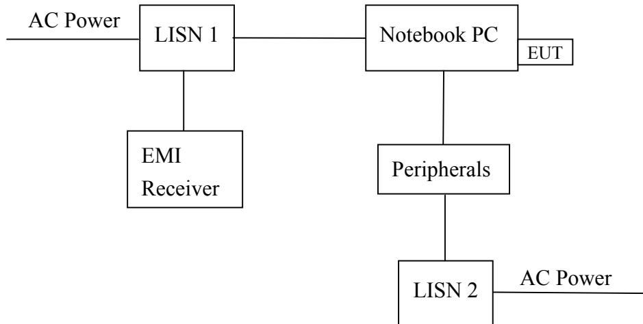
The EUT are connected to the main power through a line impedance stabilization network (LISN). This provides a 50 ohm/50uH coupling impedance for the measuring equipment. The peripheral devices are also connected to the main power through a LISN that provides a 50ohm/50uH coupling impedance with 50ohm termination.
