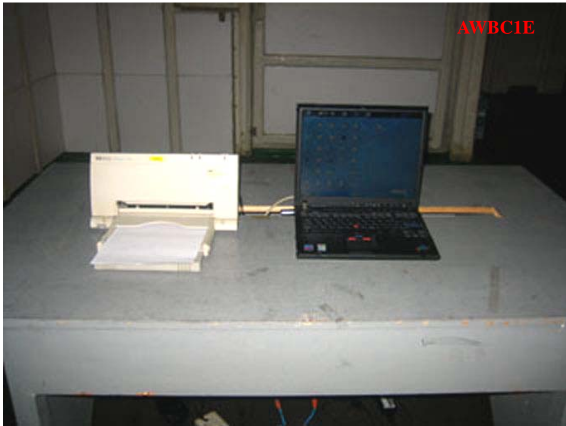
Photo 1: Radiated Emission Test set-up photo
