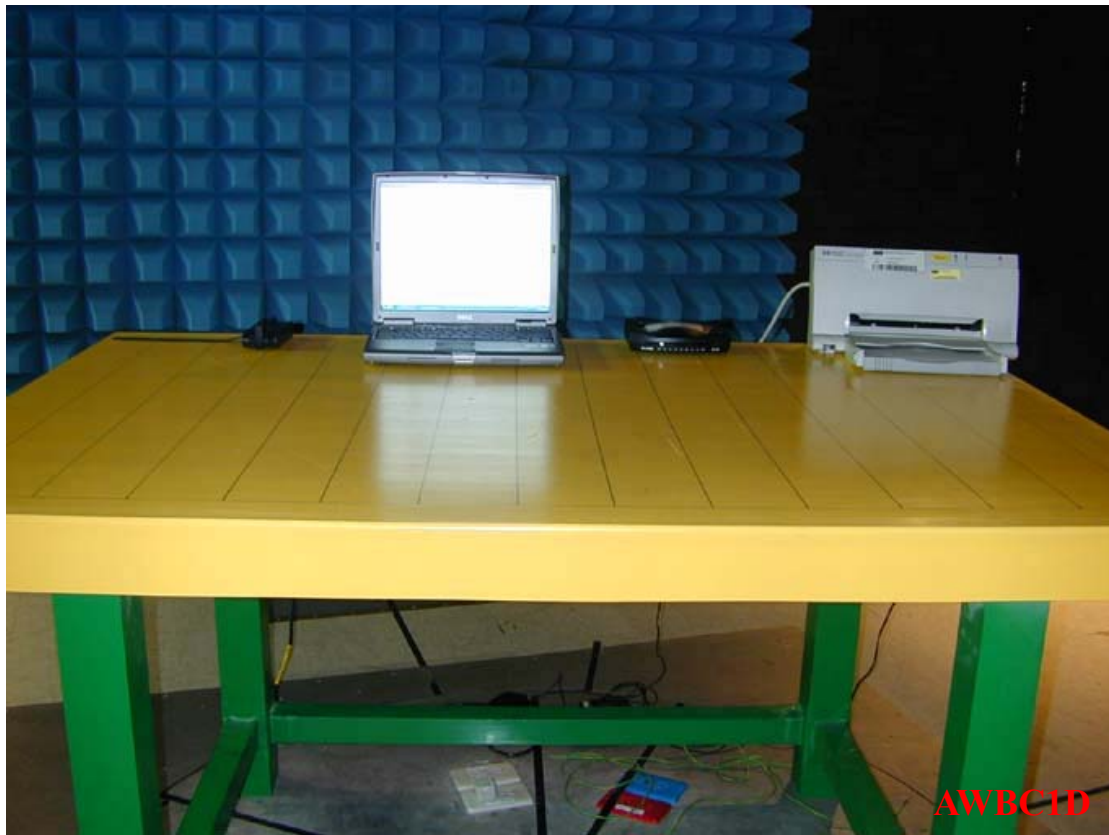
Photo 1: Radiated Emission Test set-up photo
