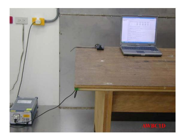
**Photo 2: Conducted Emission Test Set-up photo**
