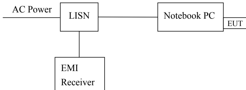
The EUT are connected to the main power through a line impedance stabilization network (LISN). This provides a 50 ohm/50uH coupling impedance for the measuring equipment. The peripheral devices are also connected to the main power through a LISN that provides a 50ohm/50uH coupling impedance with 50ohm termination.
