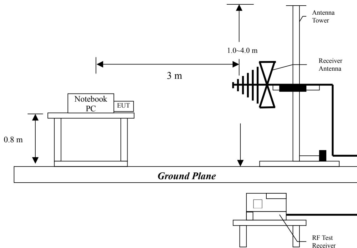
Radiated emissions were investigated over the frequency range from 30MHz to 1000MHz using a receiver RBW of 120kHz record QP reading, and the frequency over 1GHz using a spectrum analyzer RBW of 1MHz and 10Hz VBW record Average reading. (15.209 paragraph), the Peak reading (1MHz RBW/VBW) recorded also on the report.
