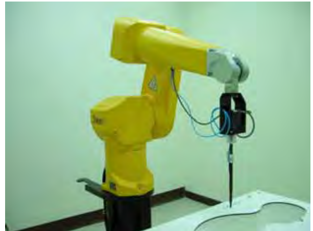
Fig. 5.2 Probe setup on robot
