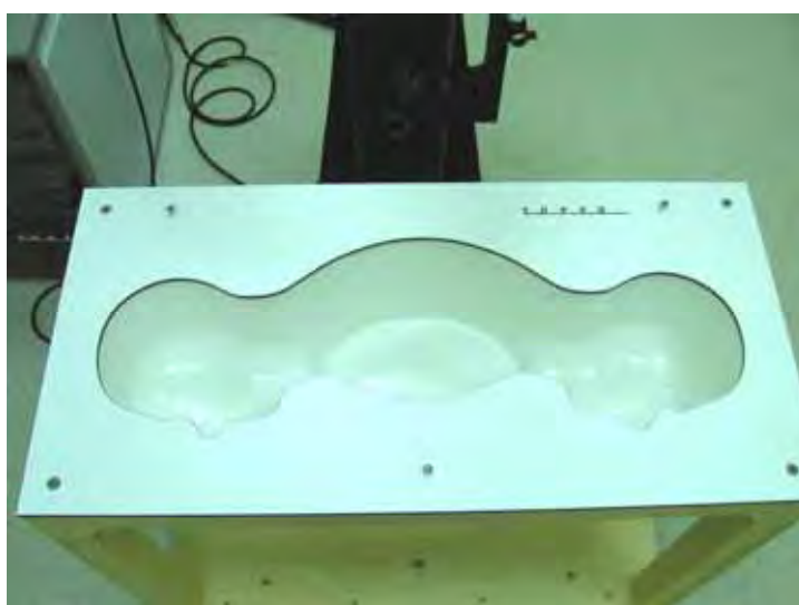
Fig. 5.3 Top view of twin phantom
