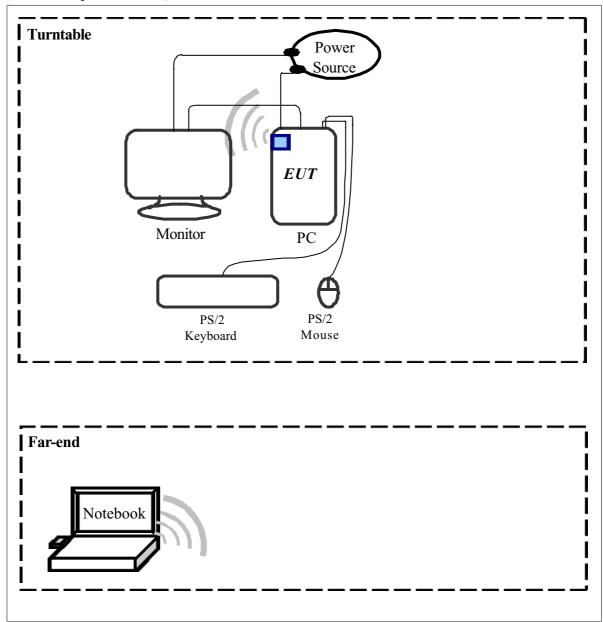
The tests below are carried out the EUT transmitter set at high power in TDD mode. The EUT is needed to force selection of output power level and channel number.
