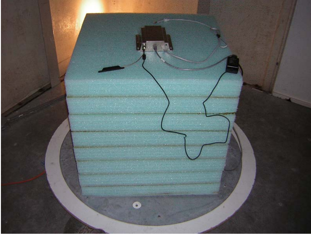
Radiated Emissions – Miltope antenna PN: 901167-1
