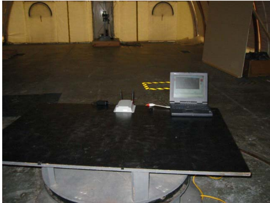
Radiated Spurious Test Setup, Front View
