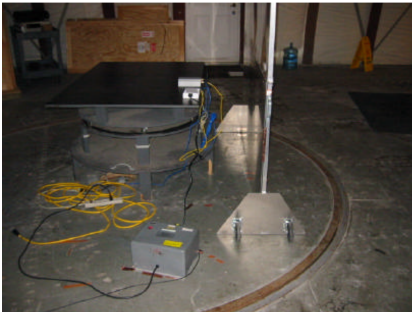
Power over Ethernet Conducted Spurious Test Setup, Side View
