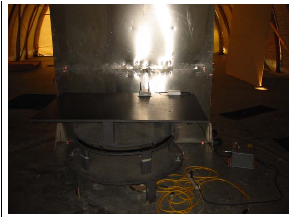
Figure 4.4-3 Conducted Emission Front View, FCC & ETSI EN 301 489-1 120V and 230V Power over Ethernet
