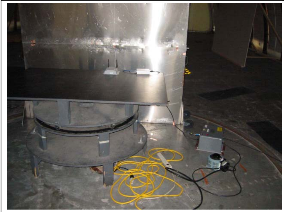
Figure 4.4-7 Conducted Emission Front View, VCCI Power over Ethernet 100V
