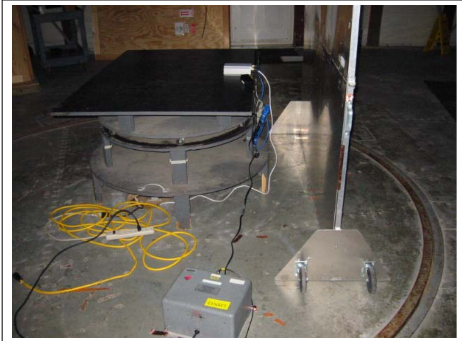
Figure 4.4-2 Conducted Emission Rear or Side View, FCC & ETSI EN 301 489-1 120V and 230V Power Supply
