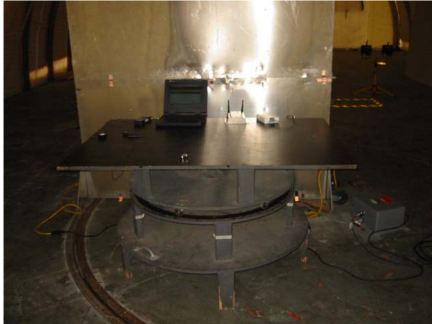
Power over Ethernet Conducted Spurious Test Setup, Front View
