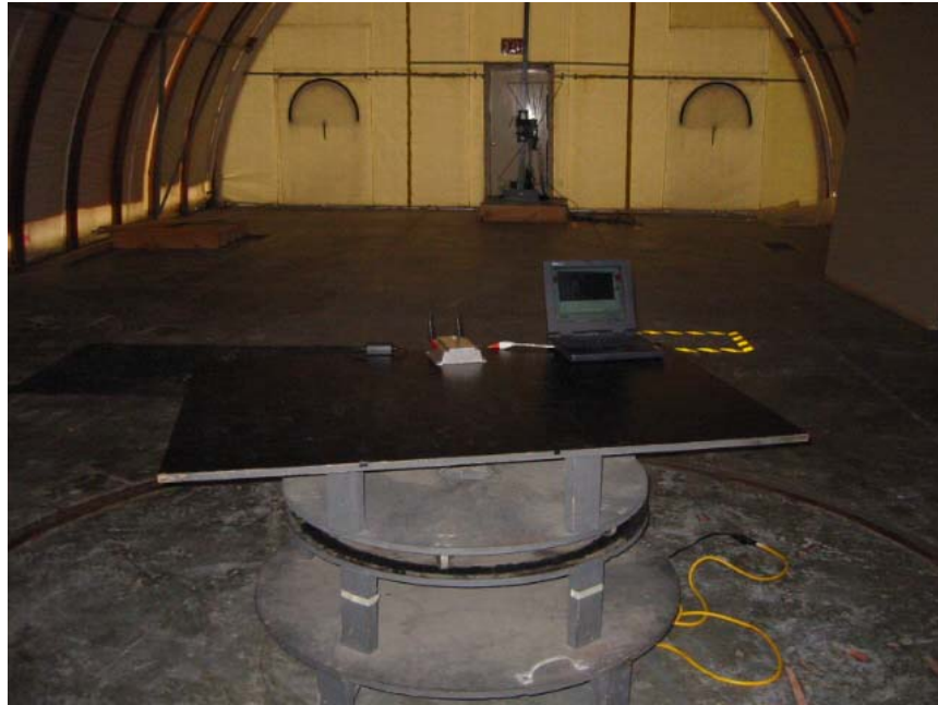
Radiated Spurious Test Setup, Front View
