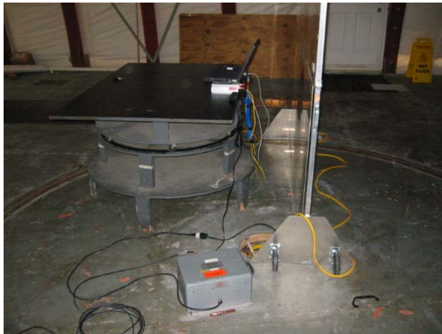
Power Supply Conducted Spurious Test Setup, Side View
