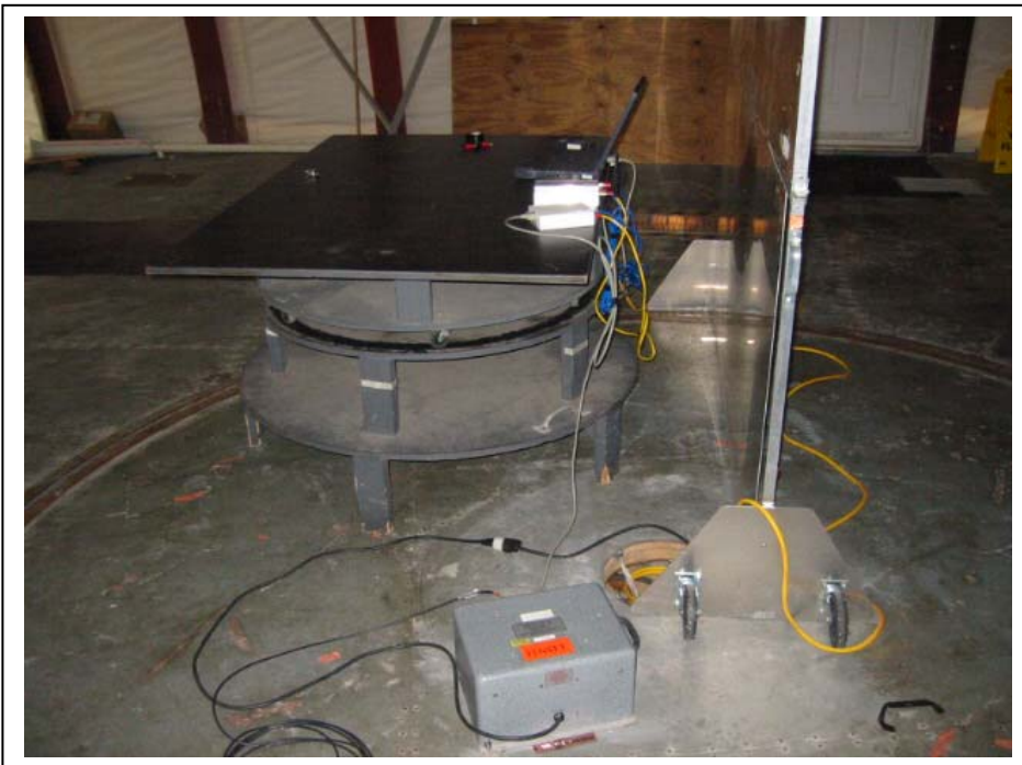
Figure 4.4-4 Conducted Emission Rear or Side View, FCC & ETSI EN 301 489-1 120V and 230V Power over Ethernet
