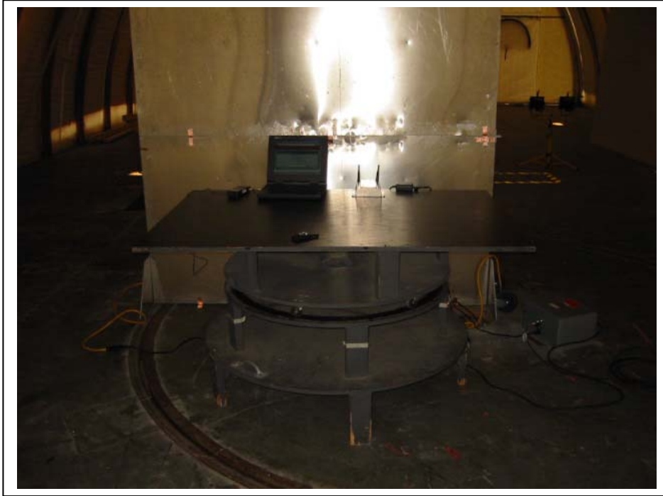
Figure 4.4-1 Conducted Emission Front View, FCC & ETSI EN 301 489-1 120V and 230V Power Supply
