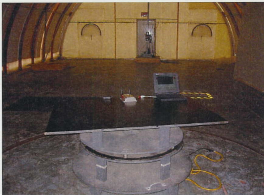
Radiated Spurious Test Setup, Front View
