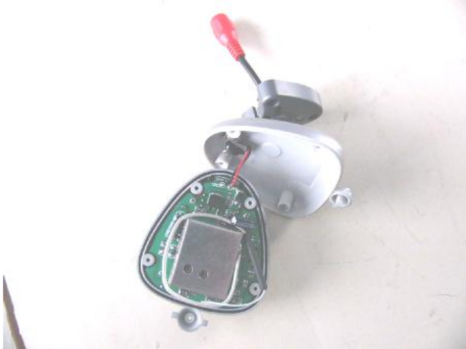
Main & RF board component side
