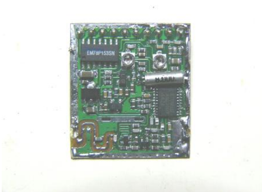
Main & RF board solder side
