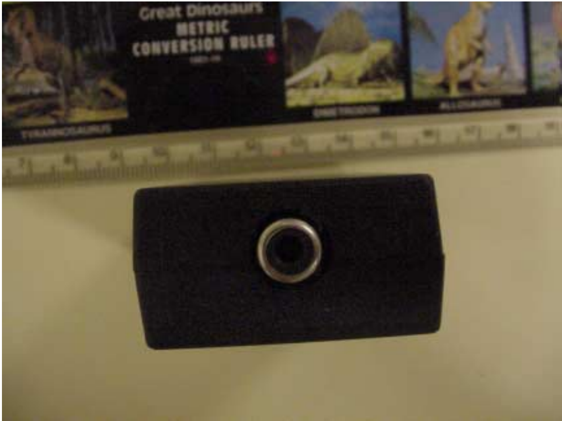
End of EUT showing RCA connector
