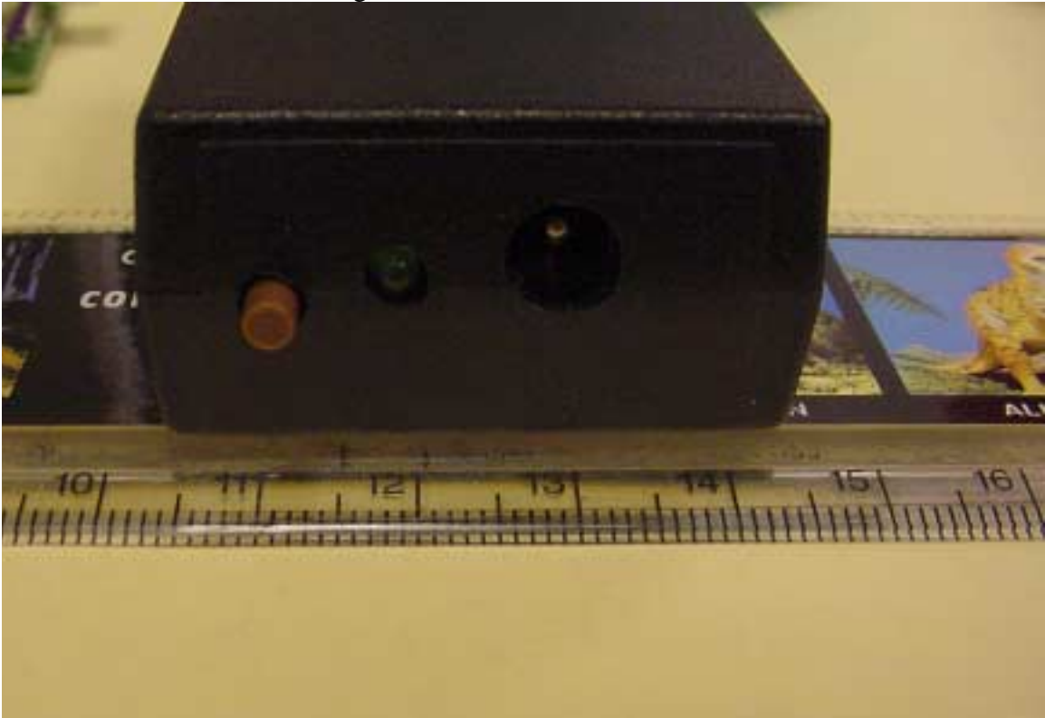
End of EUT showing channel selector switch and power entry connector.
