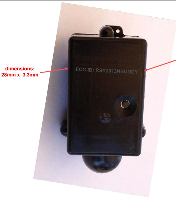
FCC ID Code engraved on the bottom of the housing
