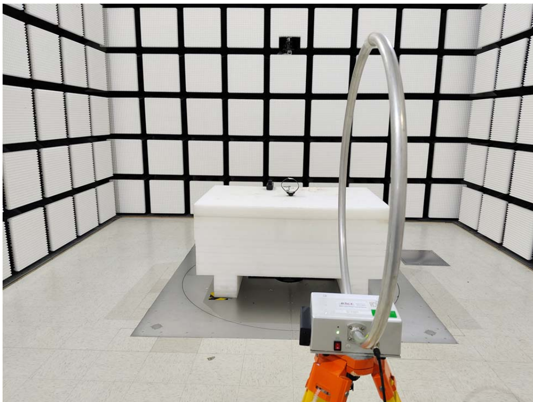
Radiated Emission 9 kHz-30 MHz Perpendicular View
