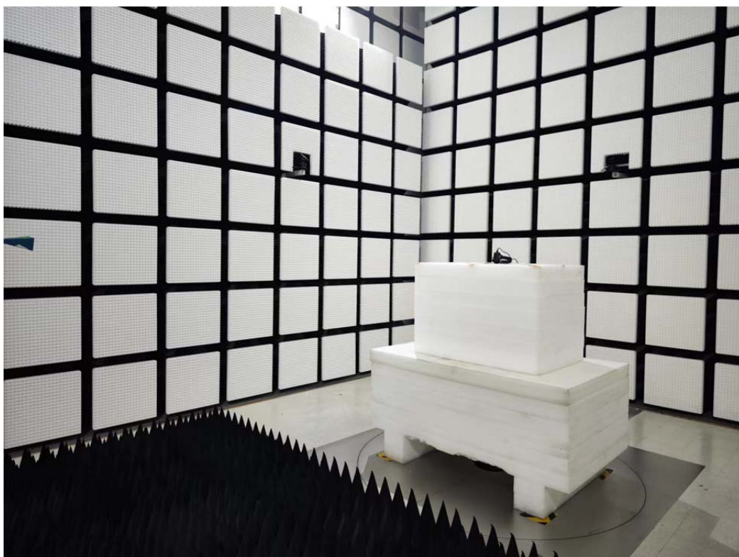
Radiated Emission Above 18-25GHz View
