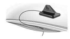
Run the cable to the inside of the vehicle near the planned location of the booster (under the seat of the vehicle, or in the front or middle console).
