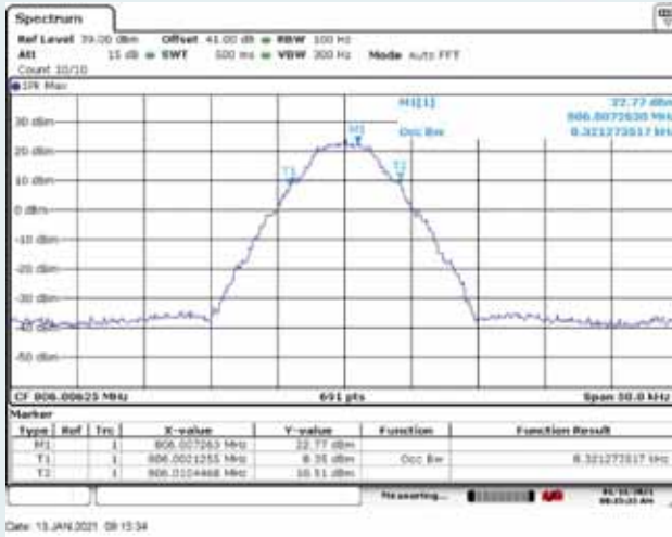
Low Frequency: 806.00625MHz, Output occupied BW (with the input signal amplitude set 3 dB above the AGC threshold)
