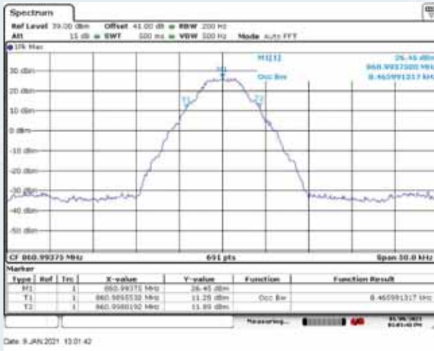
High Frequency: 860.99375MHz, Output occupied BW (with the input signal amplitude set 3 dB above the AGC threshold)
