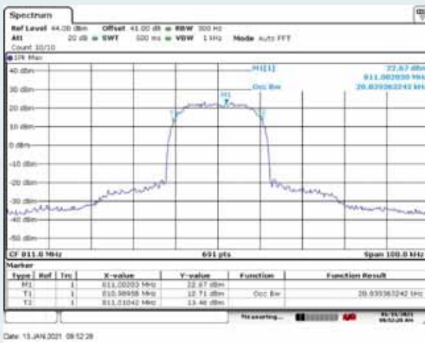
Middle Frequency: 811.0MHz, Output occupied BW (with the input signal amplitude set 3 dB above the AGC threshold)
