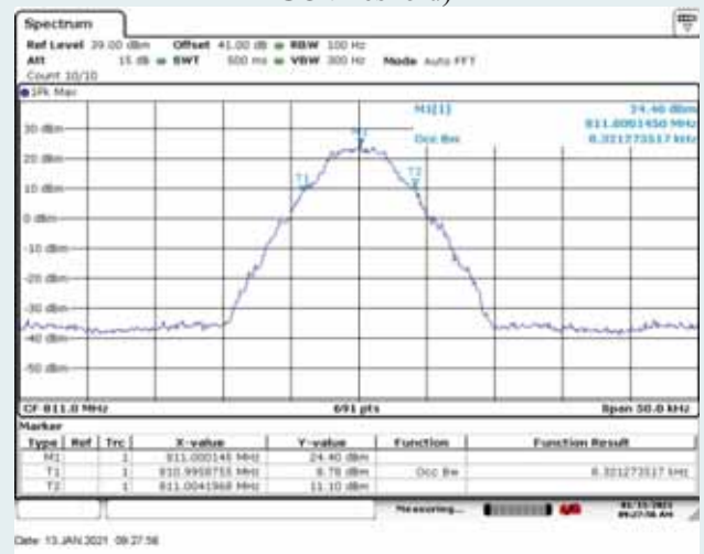
Middle Frequency: 811.0MHz, Output occupied BW (with the input signal amplitude set 3 dB above the AGC threshold)
