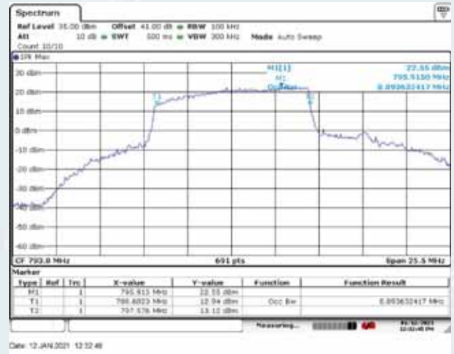
Frequency: 793.0MHz, Output occupied BW (with the input signal amplitude set 3 dB above the AGC threshold)
