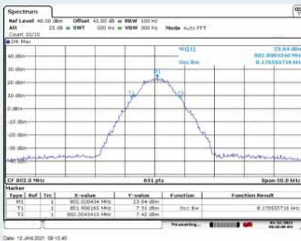
Middle Frequency: 802.0MHz, Output occupied BW (with the input signal amplitude set 3 dB above the AGC threshold)
