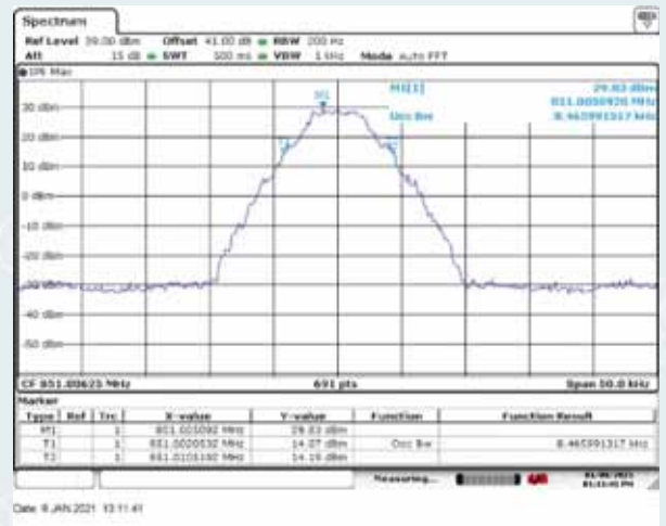
Low Frequency: 851.00625MHz, Output occupied BW (with the input signal amplitude set 3 dB above the AGC threshold)
