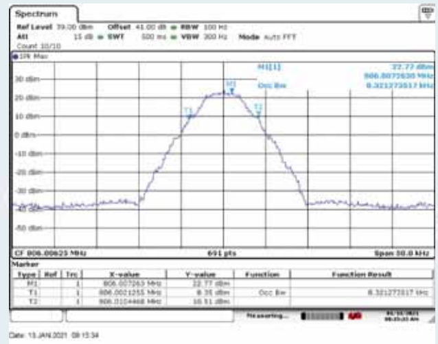
Low Frequency: 806.00625MHz, Output occupied BW (with the input signal amplitude set 3 dB above the AGC threshold)
