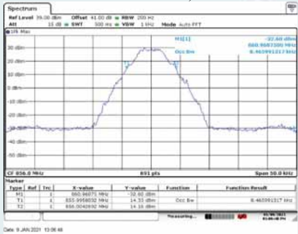
Middle Frequency: 856.0MHz, Output occupied BW (with the input signal amplitude set 3 dB above the AGC threshold)
