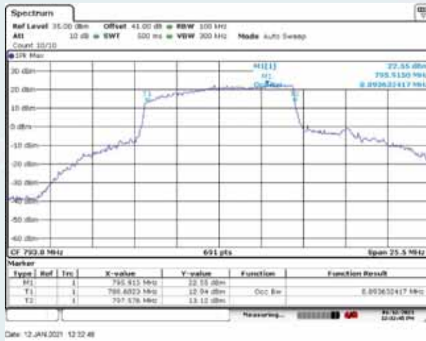
Frequency: 793.0MHz, Output occupied BW (with the input signal amplitude set 3 dB above the AGC threshold)
