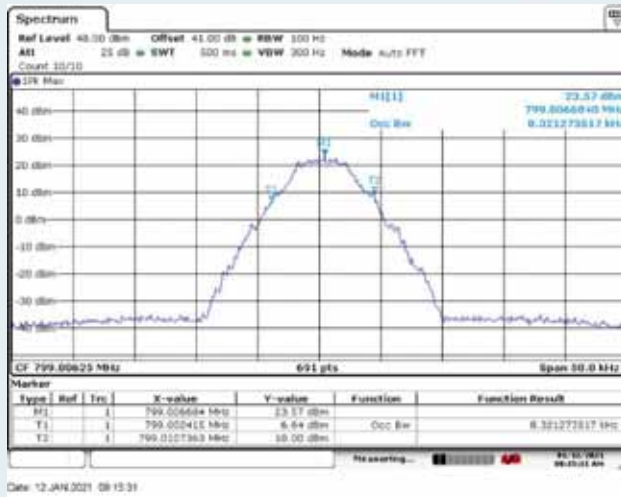
Low Frequency: 799.00625MHz, Output occupied BW (with the input signal amplitude set 3 dB above the AGC threshold)
