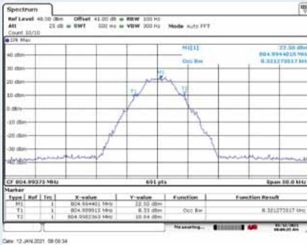
High Frequency: 804.99375MHz, Output occupied BW (with the input signal amplitude set 3 dB above the AGC threshold)
