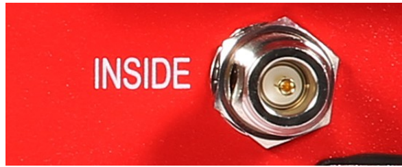
A5 — N-type Female for INSIDE cable and antenna
