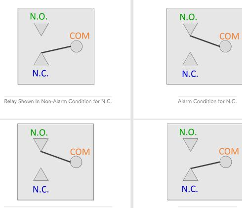
Relay Shown In Non-Alarm Condition for N.O.
