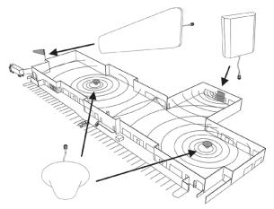
Dome antennas provide 360-degree hemispherical coverage suitable for mostly square areas, while flat panel antennas provide a focused zone of coverage suitable for long narrow areas. The example above uses two dome antennas and one panel antenna to provide full coverage
