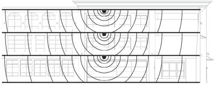
Note: You may not need antennas on every floor of a multistory building, depending on factors such as building material, BDA gain, etc.
